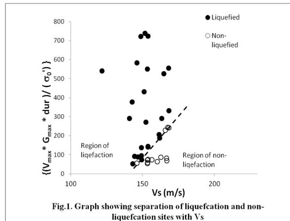
Fig.1: Graph showing separation of liquefaction and non-liquefaction sites with Vs
